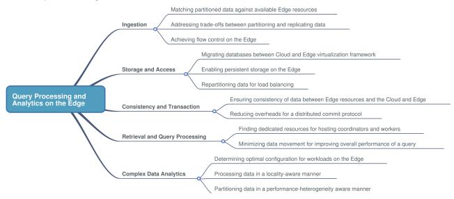
Figure 2: Challenges in developing software systems for query processing and performing data analytics on the Edge
