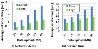
Figure 4: Network delay and service time of a sample query processing application at the Cloud and Edge
