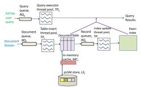
Figure 1: System architecture
