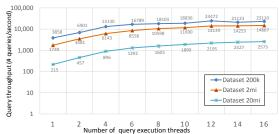
Figure 6: Query throughput (multi-threaded scalability)
