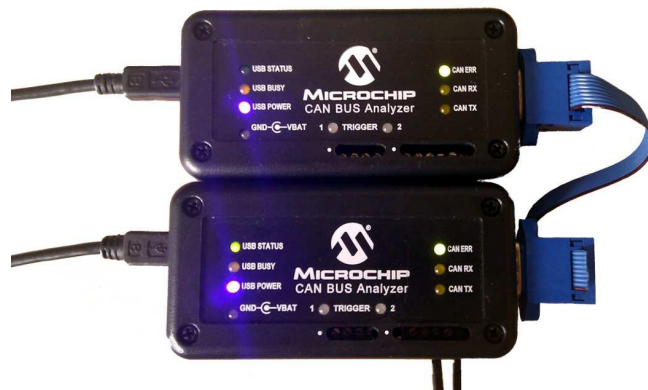
Figure 4.2: The Microchip CAN BUS Analyzer Tool [23].
