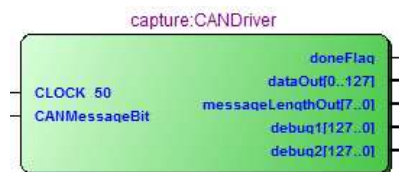
Figure 5.5: The CAN driver instance in the RTL viewer.
