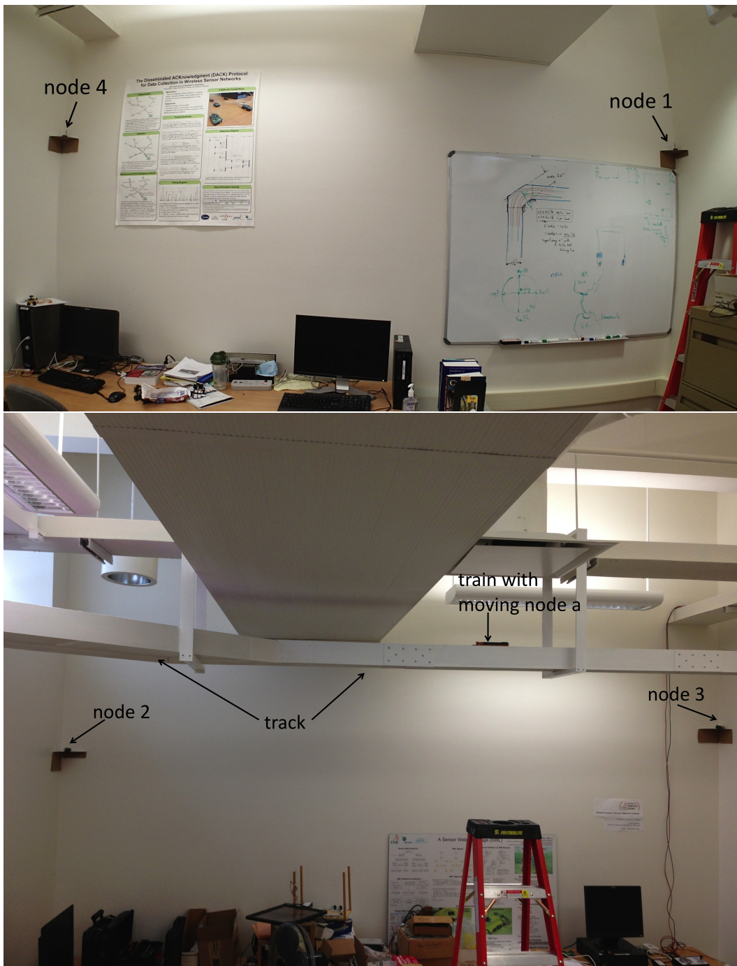
Figure 4.3: Figure (top) is the TelosB nodes deployment for static testing in ITB214 facing West and Figure (bottom) is the TelosB nodes deployment for static testing in ITB214 facing East.
