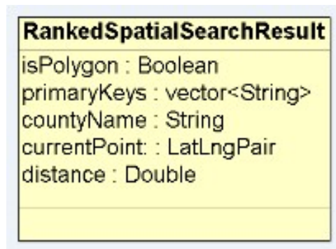
Figure 4.12: The data structure of the RankedSpatialSearchResult . Both L_1 and L_2 are stored in the structure. For L_1 results, isPolygon = “false” and countyName = \emptyset . For L_2 results, currentPoint = \emptyset .
