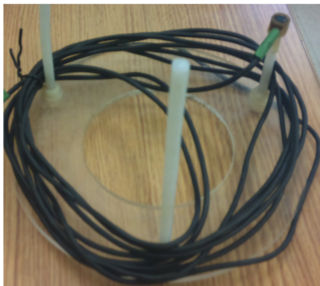
Figure 5.3: Solar Radiation sensor encased in epoxy and mounted on top of a circular rod.
