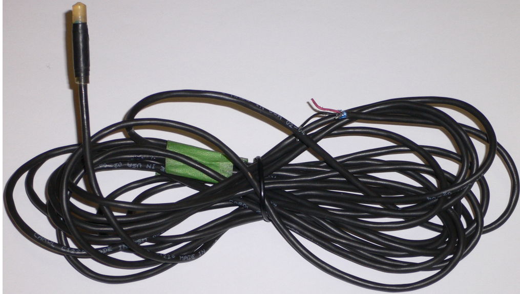
Figure 5.1: Air temperature sensor with thermistor embedded in epoxy and attached to a shielded cable.
