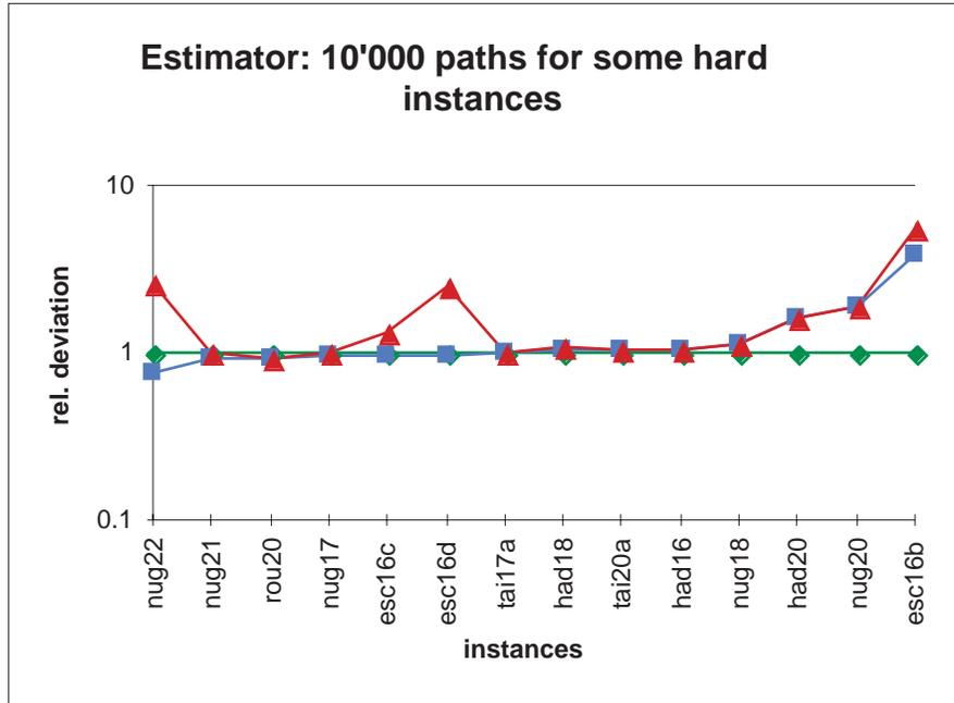
Figure 3: The parallel Branch and Bound evaluates an almost constant number of nodes when varying the number of processors.
