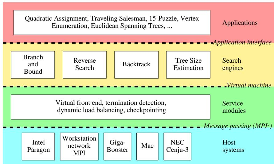
global set of work units. For Branch and Bound, a work unit is a subtree represented by its root node. Every processor repeatedly removes a work unit from the global set, does whatever work it has to do, and inserts zero or more new smaller work units into the set. When the virtual machine detects that the set is empty, the algorithm terminates.
