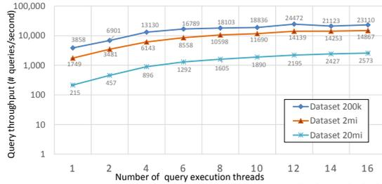
**Figure 6: Query throughput (multi-threaded scalability)**
