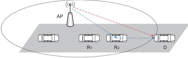
Fig. 1. System model of drive-thru Internet access with V2V relay.
