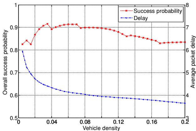
Fig. 4. Overall success probability and average packet delay with modulations adapted with vehicle density.
