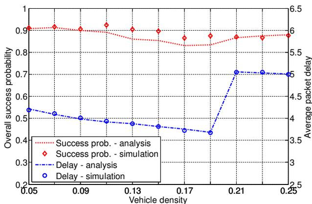
Fig. 3. Analysis and simulation results of overall success probability and average packet delay.
