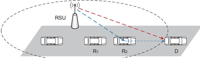
Fig. 1. System model with V2V relay.
