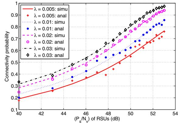
Fig. 6. Connectivity probability vs.  $(P_s/N_v)$  of RSUs.
