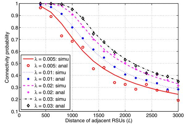
Fig. 5. Connectivity probability vs. distance of adjacent RSUs.
