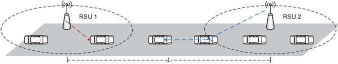
Fig. 2. Connectivity via nearby RSUs or relay vehicles.
