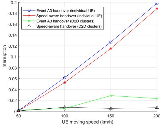
Fig. 5. Interruption probability with different handover algorithms.
