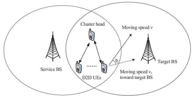
Fig. 2. Joint handover scenario with D2D cluster.
