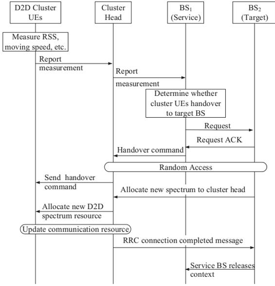
Fig. 3. Flow chart of the joint handover approach with D2D clusters.
