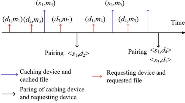
Fig. 2. Periodical processing of D2D pairing.
