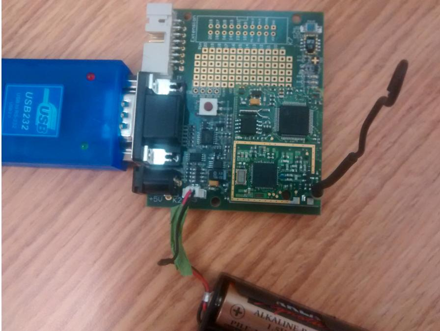
Figure 2: Tinynode 584 with standard extension board with a battery pack and serial connection to the computer.
