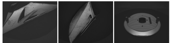
Fig. 1. Paint inspection images obtained with deflectometry inspection technology for three different objects.
