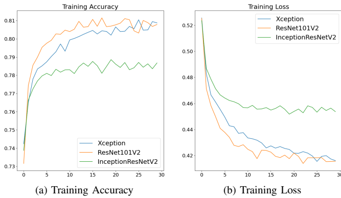
Fig. 5. Results of feature extraction accuracy and loss for the transfer learning models
