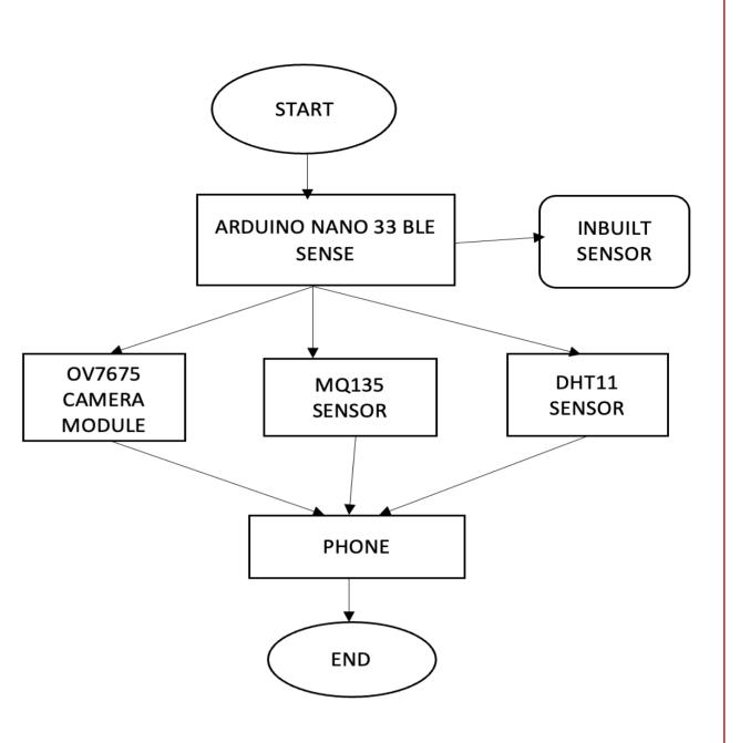
The flow chart explains the process of collecting data using the sensor. The proposed system uses Arduino Nano 33 BLE Sense, a board with multiple inbuilt sensors. This board is connected to an OV7675 camera module, an MQ135 sensor and a DHT11 sensor. This connection is attached to a shield board, and the real-time data is displayed on a mobile screen.
