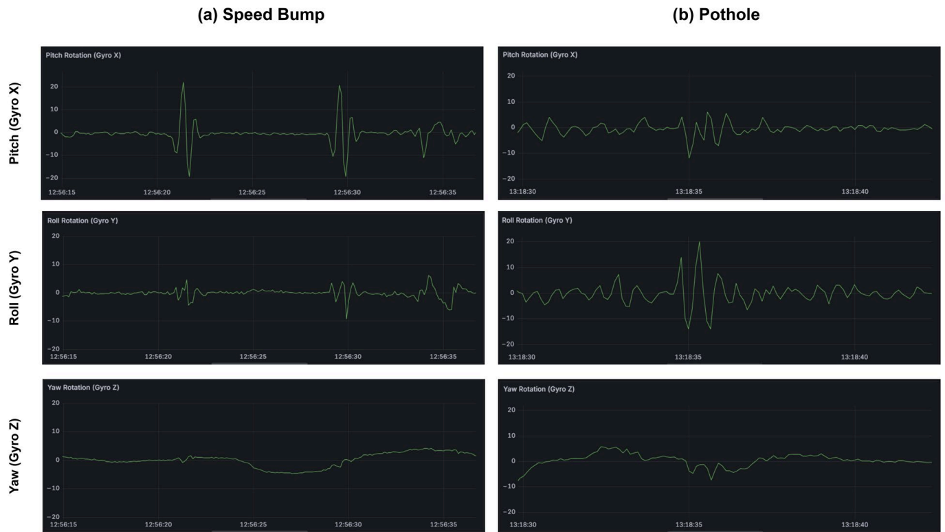
Figure 14. Gyroscope responses of SN #1 during (a) a speed bump and (b) a pothole event.
