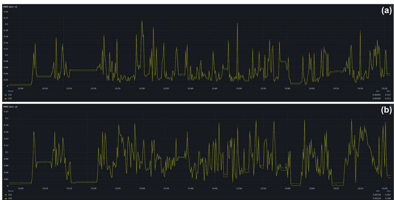
Figure 11. RMS acceleration in the (a) lateral (X) and (b) longitudinal (Y) directions for both sensing nodes.
