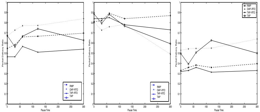
**Fig. 1.** Attraction-point packet delivery ratio for OLSR and AODV and ZRP
