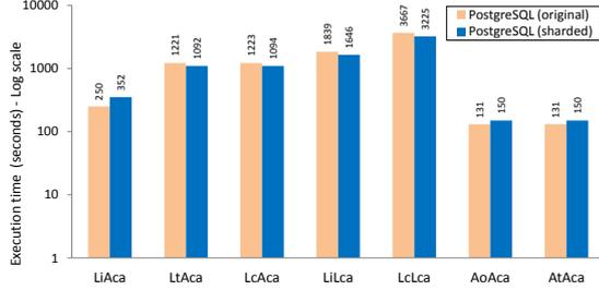
Figure 7: Query execution times - original vs Sharding-StoredProc (California dataset)
